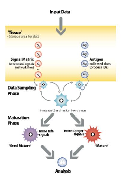
Figure 4: Schematic overview of the DCA.
