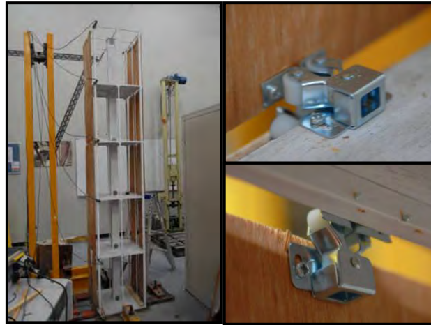
Figure 6-27 Details of the double roller connection of infill panels to the frame
