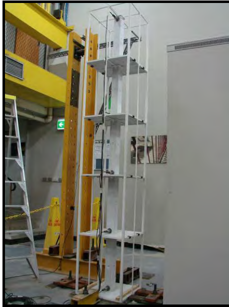
Figure 6-16 Cables of accelerometers are attached to the frame along the loading direction
