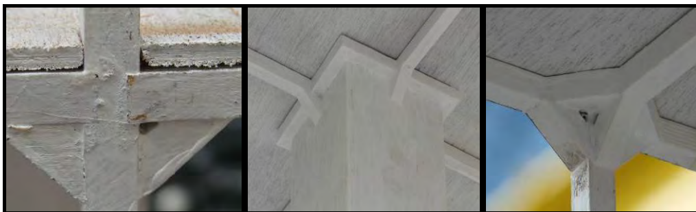
Figure 6-3 Connection details of the laboratory model
