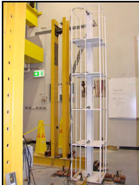
Figure 6-17 Cables of accelerometers are attached to the frame across the loading direction
