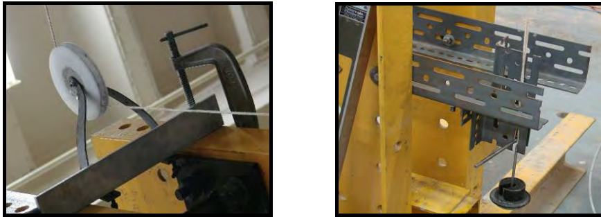
Figure 6-26 Loading system, crown block and the weights
