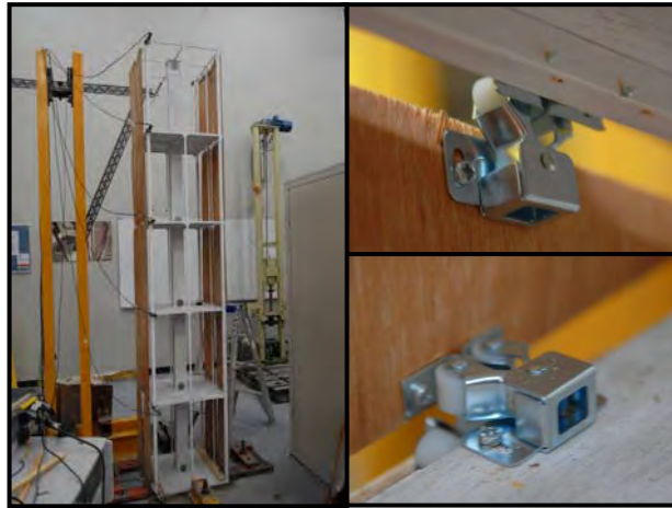
Figure 6-4 Details of the double roller connection of infill panels to the frame
