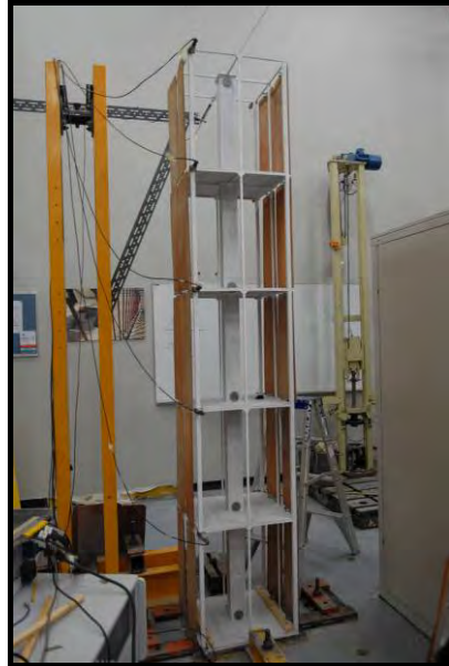
Figure 6-18 Cables of accelerometers were hung up to a freestanding steel post
