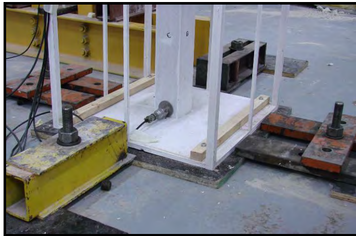
Figure 6-5 Bottom fixing details of the laboratory model
