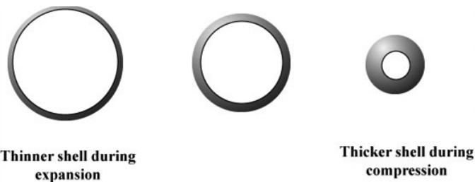
Figure 4: A depiction of the change in mass transfer boundary layer (shell) thickness of a bubble during the expansion and compression cycles of an acoustic wave. The concentration gradient is thus enhanced during bubble expansion.
