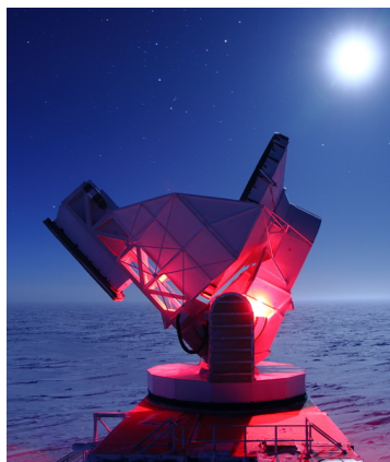
Fig. 1. The 10-m South Pole Telescope. The first camera, SPT-SZ, observed from 2007-2011. The cluster catalog in this talk is from the SPT-SZ survey. The second polarization-sensitive camera, named SPTpol, is currently observing. A third camera, SPT-3G, with ten times more detectors than SPTpol is slated to begin observations in early 2017.
