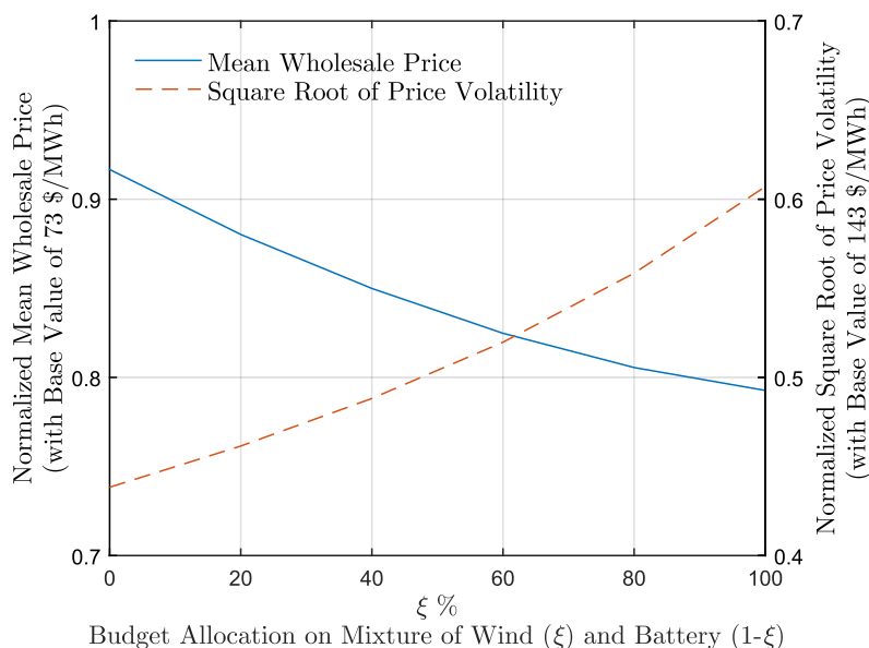
Figure 6.4: Normalized mean wholesale price and square root of price volatility for different mixtures of regulated wind and regulated battery with the equivalent annual budget of 300 m$ in VIC.
