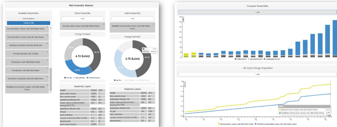
Figure 5. Assembly selector analysis page displaying results of edited assembly compared to the original assembly (left), other assemblies (top right) and life cycle energy projection (bottom right).
