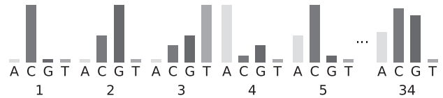
Fig. 4. Schematic representation of phasing in Illumina Solexa sequencing. The figure shows intensities detected across cycle where the true sequence reads CGTAC... Cross-cycle signal leakage can be seen, for example, in cycle 2 which contains a significant fraction of the intensity present in cycle 1. By the final cycle, the signals are almost fully convolved and it becomes difficult to determine the true signal. Phasing is caused by the non-incorporation of a labelled nucleotide in a given cycle. The reverse phenomenon (data not shown) is caused by the multiple incorporation of nucleotides and manifests itself as signal leakage between the current and previous cycles.
