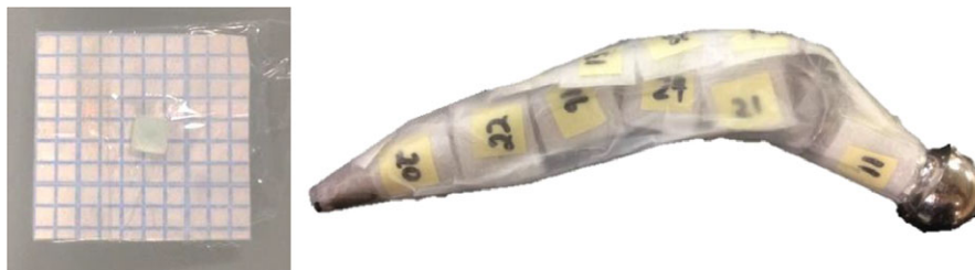
FIG. 3. The left figure shows a 3 \times 3 \text{ mm} TLD-100H chip. It is affixed to a small square of graph paper by plastic cling wrap which is held in place by double sided tape at the edges of the square. The right figure shows the graph paper squares with attached TLDs affixed to the hip prosthesis following irradiation.
