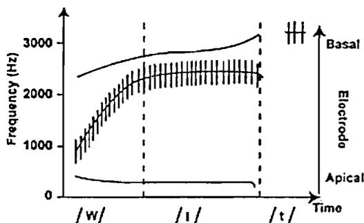
Figure 2: A diagram of the Second formant (F2)/Fundamental frequency (F0) speech processing strategy for the word /wit/.
