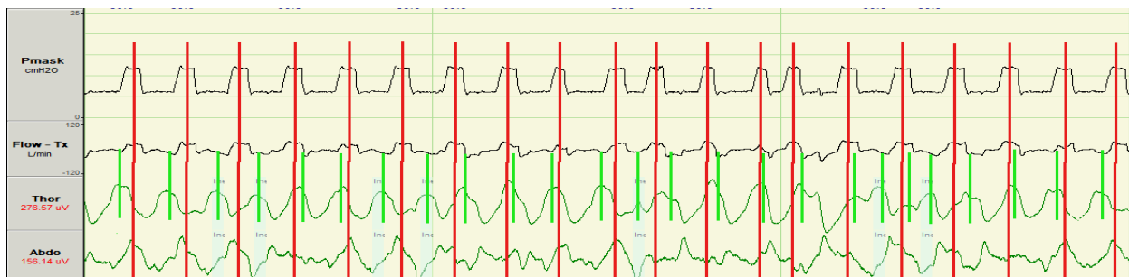
Figure 1. PVA detection of Ineffective Effort events via frequency difference detection. The red lines in the figure are lined up with mask pressure cycles, whereas the green lines are lined up with thoracic signal cycles. As we see, there are 20 Pmask cycles in this snippet, but there are 25 corresponding Thor cycles, indicating there are missed ventilation cycles.
