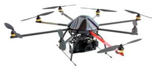
An Unmanned Aerial Vehicle (UAV) is an aircraft flown either controlled autonomously, semi-autonomously or under the remote control of a pilot on the ground or in another vehicle (See Figure 4). UAVs address the limitations of the traditional airborne-based mapping systems, including the high flight altitude which results in low resolution, inadequate for land and property information management and high cost. UAV based mapping provides the required accuracy
