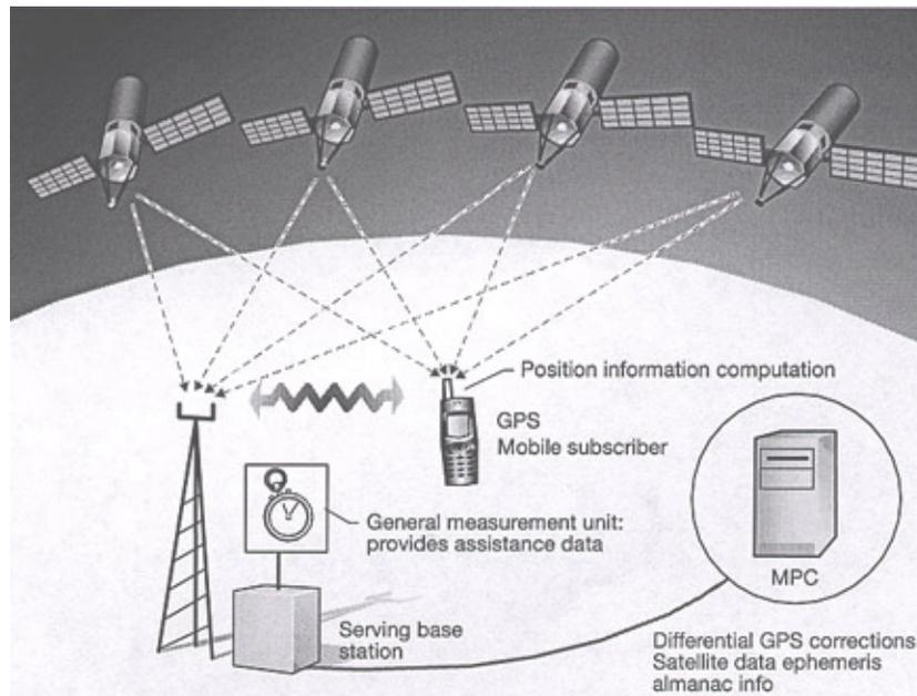
Figure 3 – Assisted GPS positioning (Swedberg, 1999)
