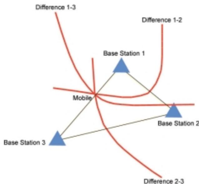
Figure 1 – Enhanced Observed Time Difference Positioning Technique
