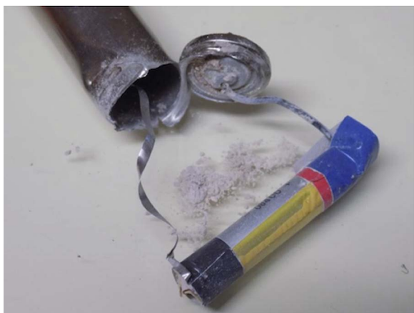
Figure 1. Opened UltraFire-labelled cell consisting of large shell with small internal cell (republished with permission from Ref. 1).
