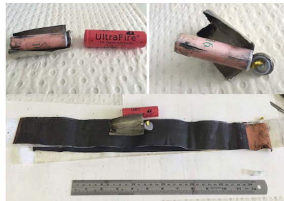
Figure 3. Opened sample of UltraFire TR18650 4200 mAh cell tested in original paper.
