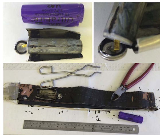
Figure 4. Opened sample of UltraFire TR18650 4900 mAh cell tested in original paper.
