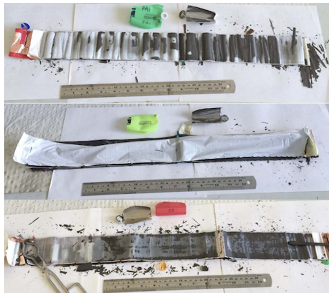
Figure 6. Opened sample of the other cells tested (from top: Panasonic NCR18650A, Panasonic NCR18650B, Sanyo UR18650FM).
