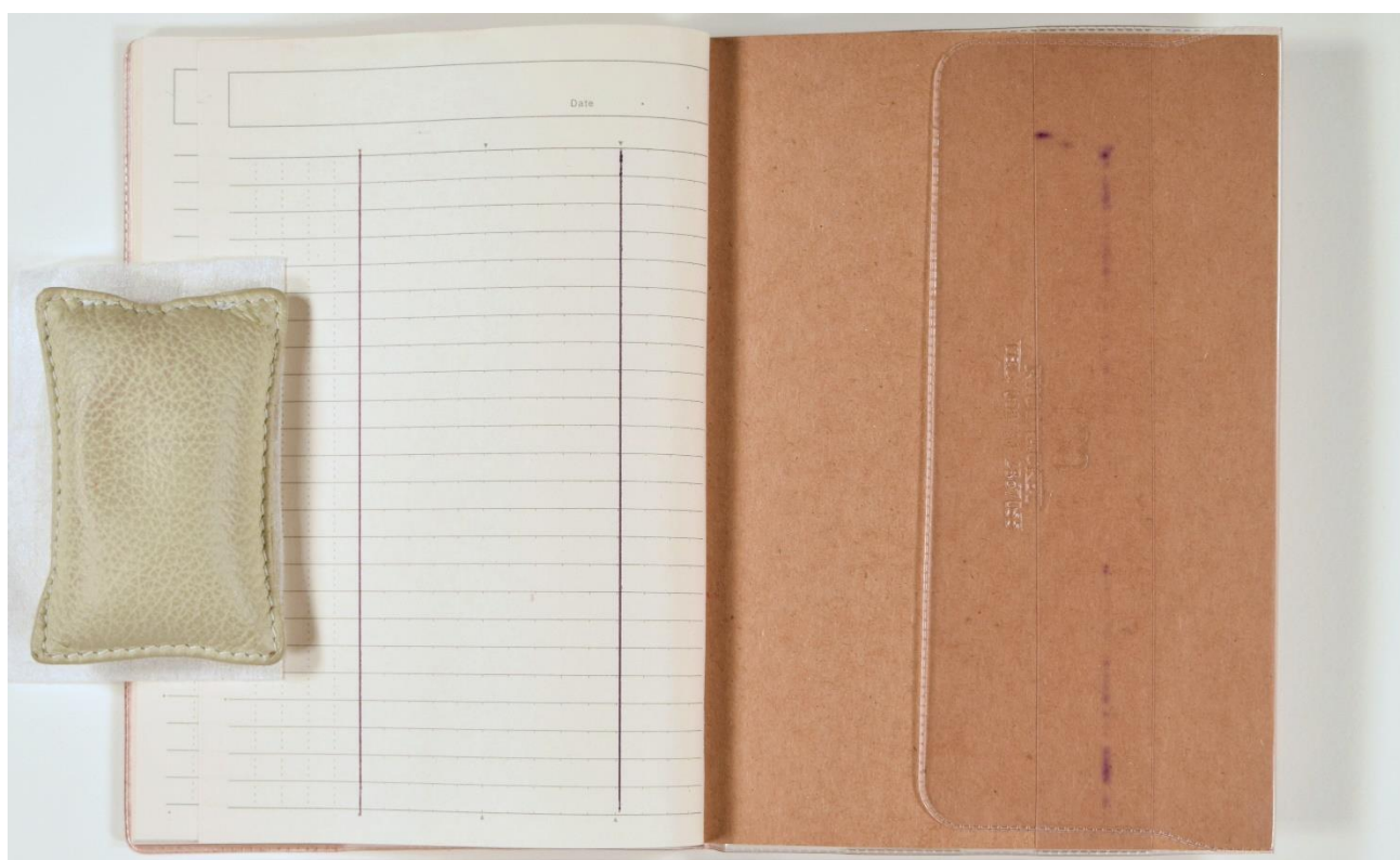
Fig. 6. Example of offsetting occurring in a non-interleaved control sample.
