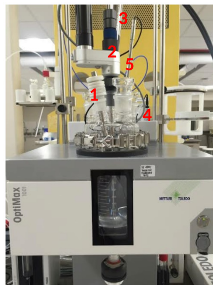
145 Figure 2: The schematic of OptiMax 1001 crystalliser equipped with temperature, heat flow and FBRM 146 sensors (left); and a photo of the crystalliser without showing the water bath and computers (b).
