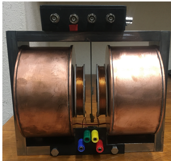
Fig. 4.3.: Photograph of the benchtop electromagnet used in the high-field EDMR setup with a sample attached to the custom-designed PCB situated at the centre between the poles of the electromagnet. Electrical contacts to the device are accessible via the four available female BNC connectors mounted on the breakout box.
