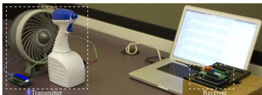
Figure 1.1: Tabletop testbed sending alcohol through space [1] © 2014 IEEE.
