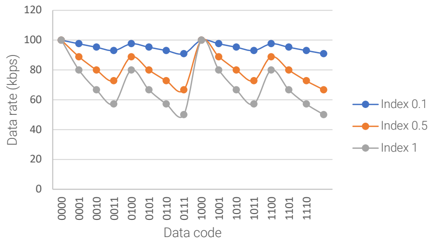
Figure 2-22 Theoretical 4-bit instantaneous data rate based on transmission code and minimum pulse width of 10us.
