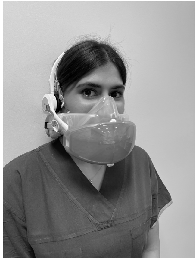
Fig. 1. A healthcare worker wearing a HALO CleanSpace powered air-purifying respirator and a wireless communication headset device.
