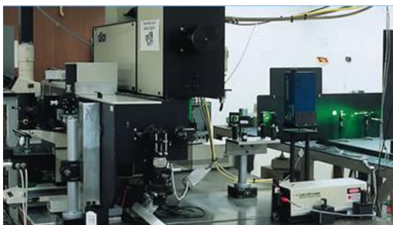
Appendix Figure 1. Dilor XY Raman Spectrometer in the School of Physics, University of Melbourne
