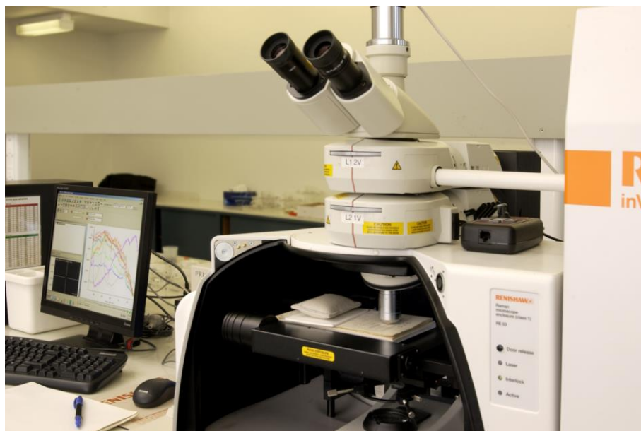
Figure 22. Streeton catalogue inside the Raman spectrometer
