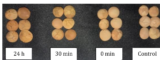
Figure 10.9 Colour change of lentil seeds treated by remote plasma with 30% air for 100 s at different holding times
