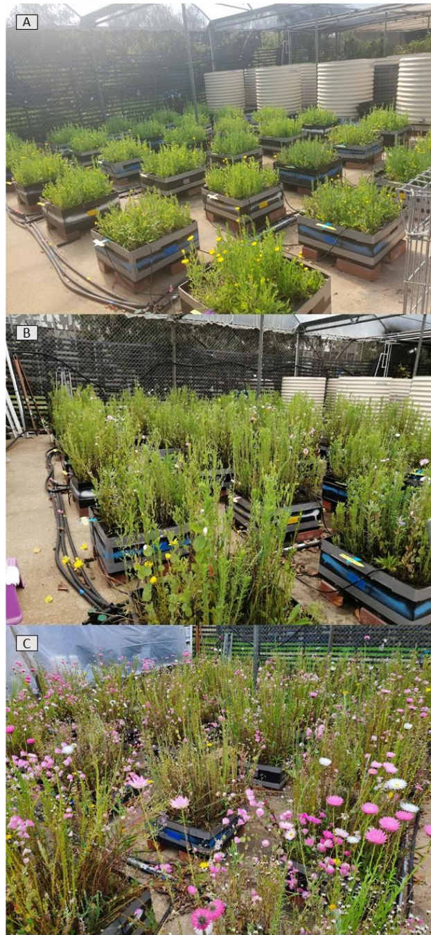
Figure 4.2. Green roof modules at the experimental site of University of Melbourne, Burnley Campus, three (A), six (B) and nine (C) months after sowing (April, July, Sep 2020, respectively).
