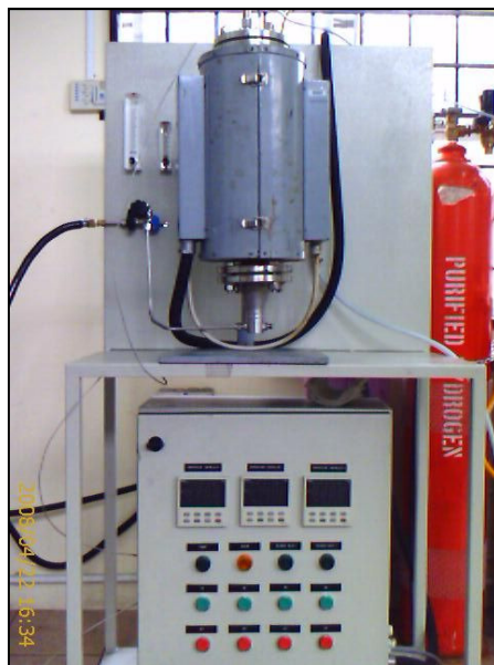
Figure 3.13 - Photograph showing the fluidised bed reactor used for palm fibre char production.
