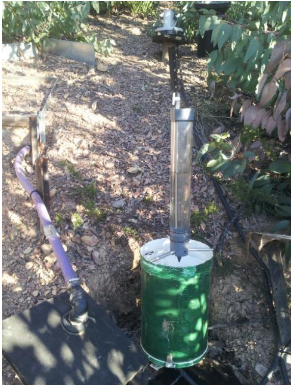
Figure 3.5 From top to down: Calibration of tipping bucket connected to runoff plots and rain gauges.
