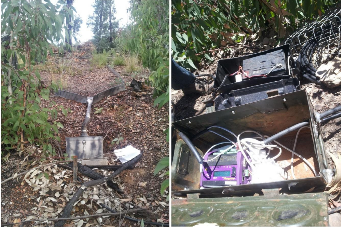
Figure 3.4 Runoff plot connected to its tipping bucket (left), Data logger connected to its battery (right)
