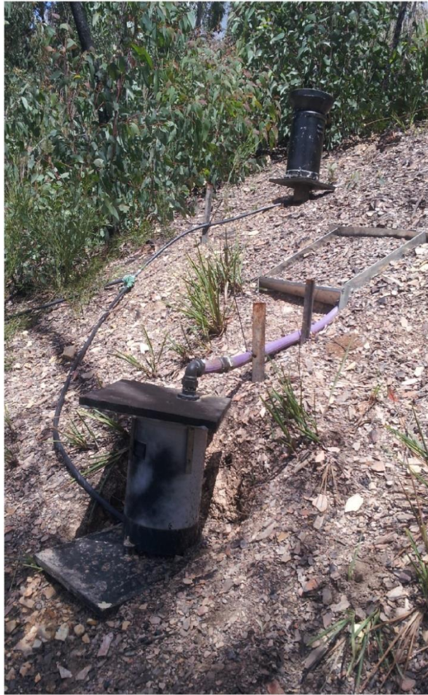
Figure 3.2 Paired rain gauge-infiltrometer
