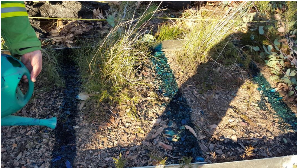
Figure 6.2 Applying blue dye solution across the transects
