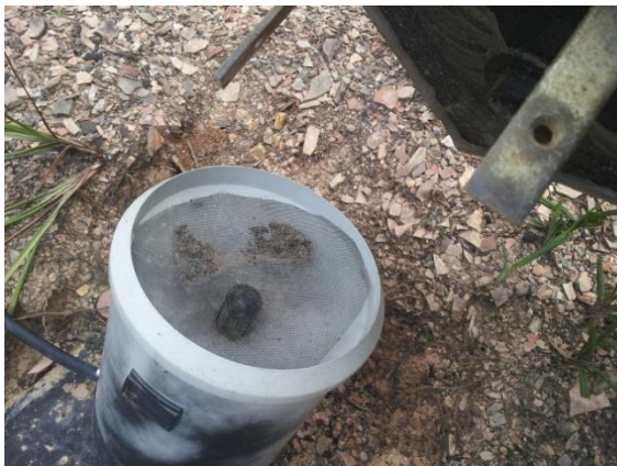
Figure 3.6 Metal mesh and fabric mesh form used to capture fine residue
