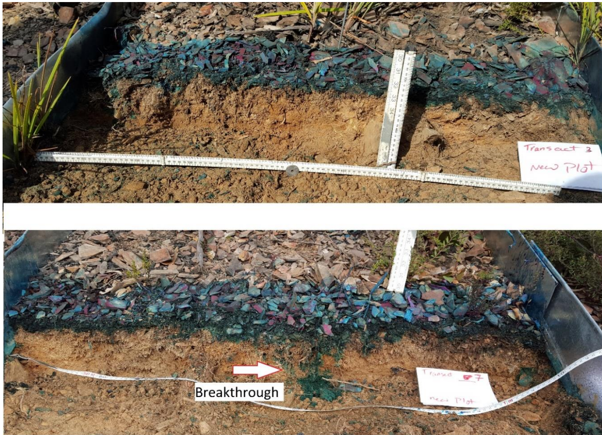
Figure 6.3 Manual measurements of preferential flow path and wetted area within vertical soil profile
