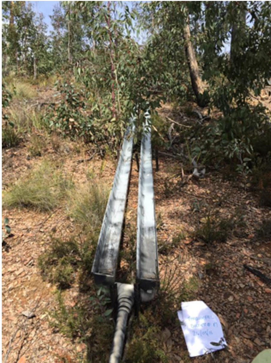
Figure 3.3 Throughfall gutters to its tipping bucket
