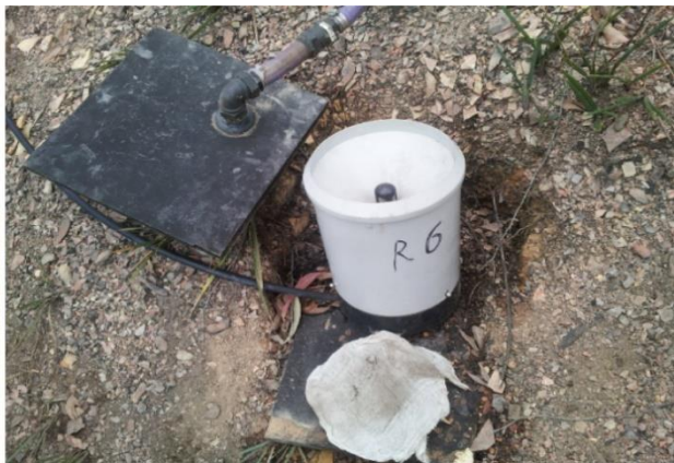
Figure 3.6 Metal mesh and fabric mesh form used to capture fine residue
