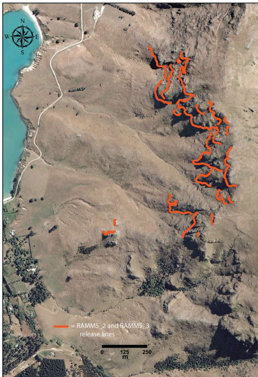
Figure A6. Polyline shapefiles for RAMMS_2 and RAMMS_3 rockfall source areas. (Image is modified after Land Information New Zealand, https://data.linz.govt.nz/data/category/aerial-photos , last access: 6 March 2019.)
