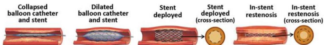
Figure 2.4 The formation of restenosis after balloon angioplasty, taken from Yin et al. (2014).
