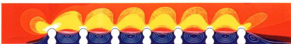
Figure 2.7 Simulation result of an early study: Shear rate contour (color) and streamline (white line) (Berry et al., 2000).
