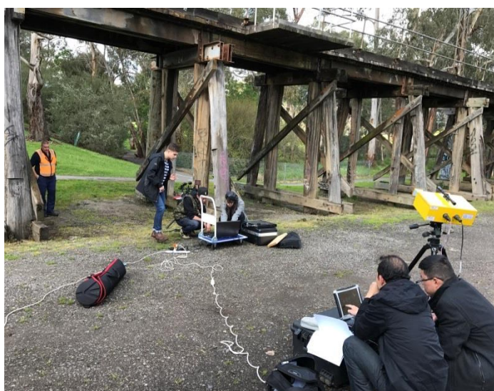
Figure 1 Structural monitoring of the bridge using IBIS-S and ARAMIS
