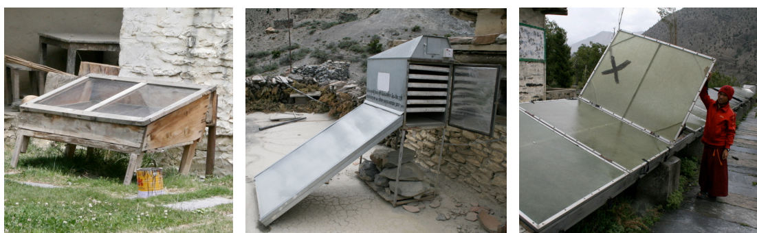
Figure 51 - Solar dryers in Lower Mustang: direct box type; indirect cabinet; large-scale tunnel dryer (photos – S Candy).
