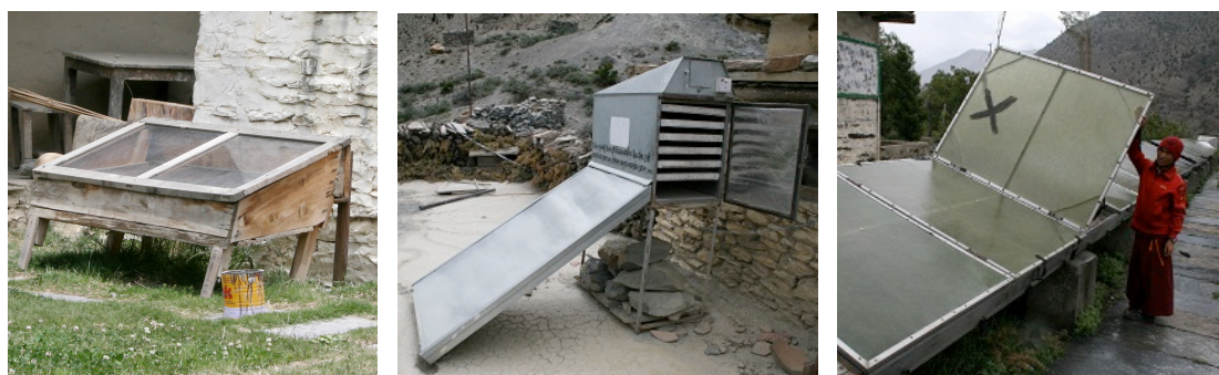
Figure 21 - Solar dryers in Lower Mustang: direct box type; indirect cabinet; large-scale tunnel dryer (photos – S Candy).
