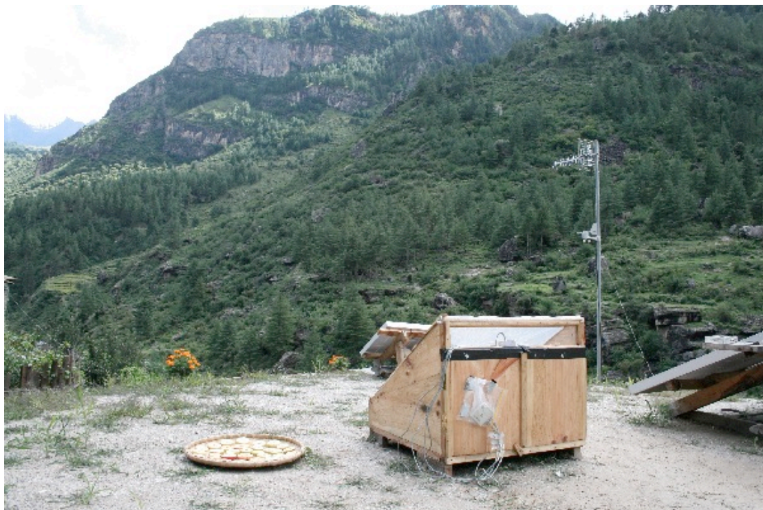
Figure 55 - Solar dryer experimental set-up in Humla (loaded test) (Photo – S Candy).
