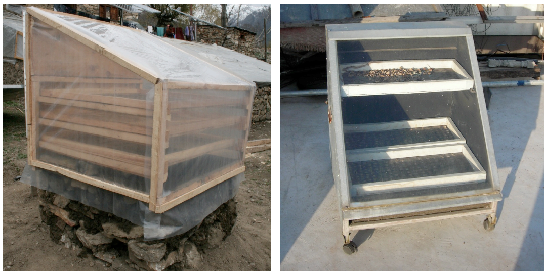
Figure 52 – Initial solar dryer design; Kathmandu solar dryer design (Photos - S Candy).
