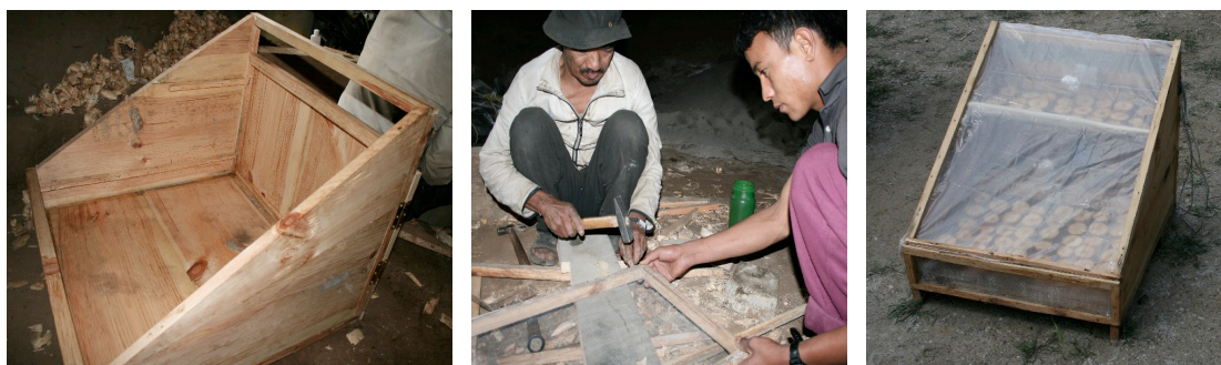
Figure 53 – Construction of the direct box type solar dryer in Humla (Photos – S Candy).
