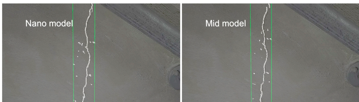
Figure 14. Example of the execution of the integrated model using the YOLO v5n (left) and YOLO v5m (right) structures in the HoloLens.
