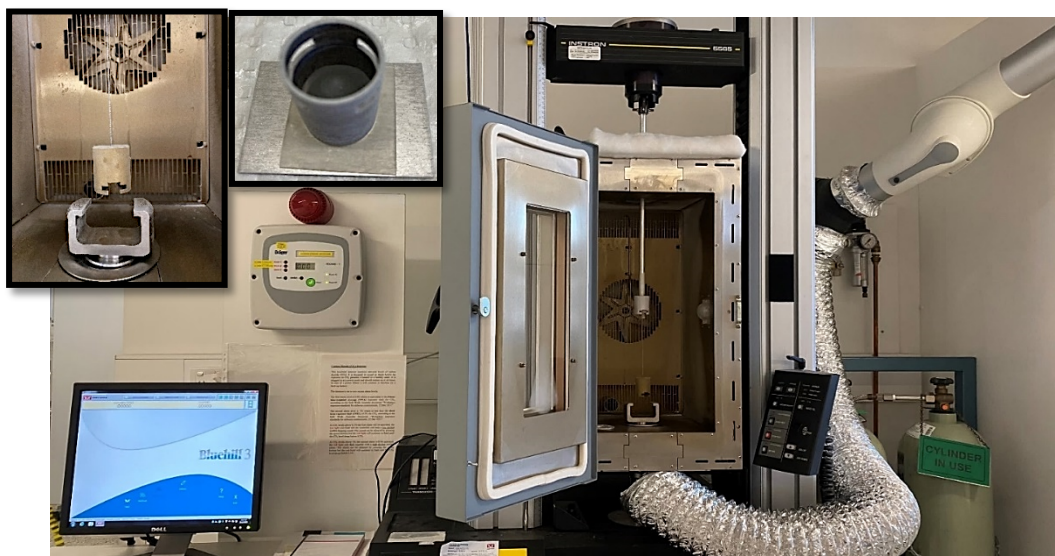
Figure S6. Ice adhesion test apparatus.
