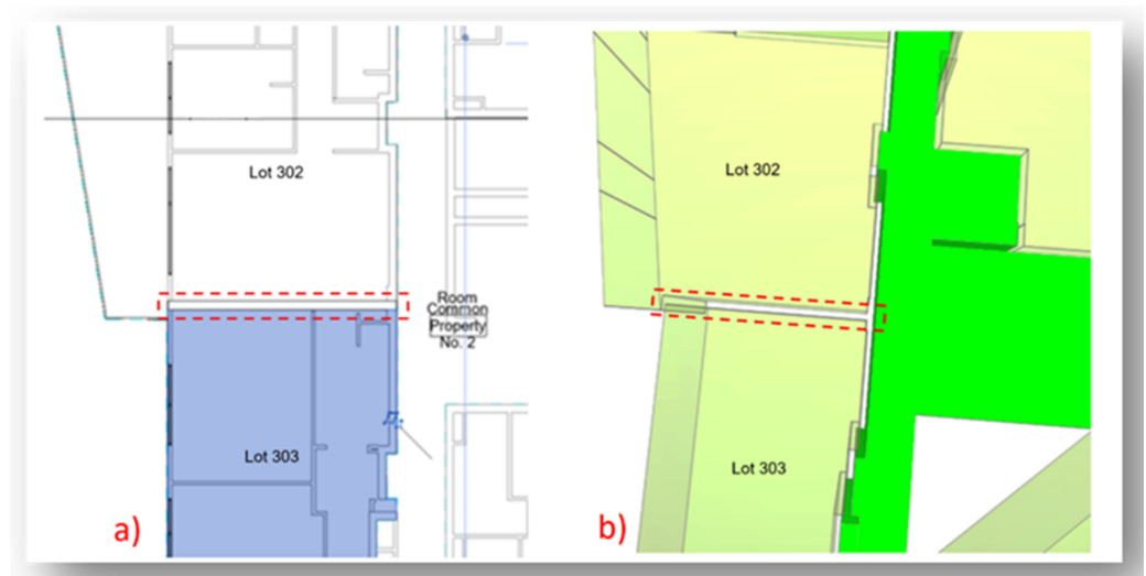
Figure 9. Errors in authoring the cadastral information stage. (a) An undefined ownership space in the BIM model, (b) a gap created in IFC data format.
