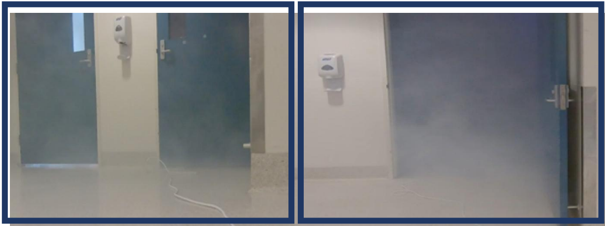
Figure S4: Comparison of smoke exiting the patient room with the door closed (left) and open (right).
