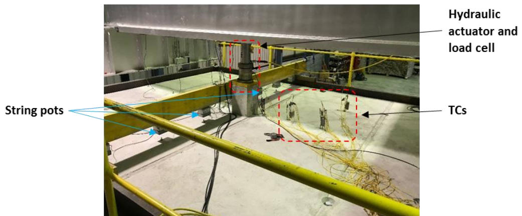
Figure 3.8: TCs, String pots and hydraulic actuator fixed to the specimen
