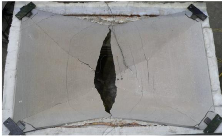
Figure 2.6 Failure mode of a simply supported RC slab at elevated temperatures (Bailey and Toh, 2007)
