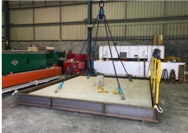
Figure 3.6: Slab specimen with the supporting frame prior to mounting on the furnace
