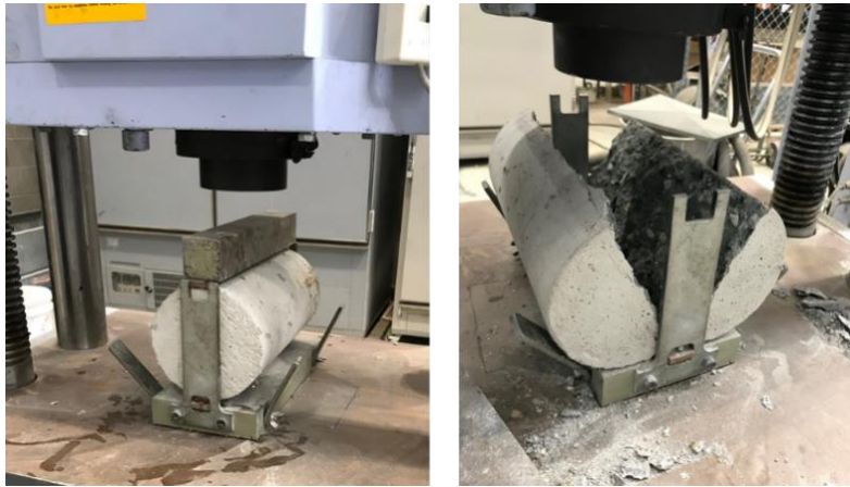
Figure 3.4: Splitting tensile test set-up and a failed specimen after the test
