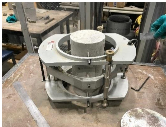
Figure 3.5: Test specimen for Young's modulus test with deformation measurement rig
