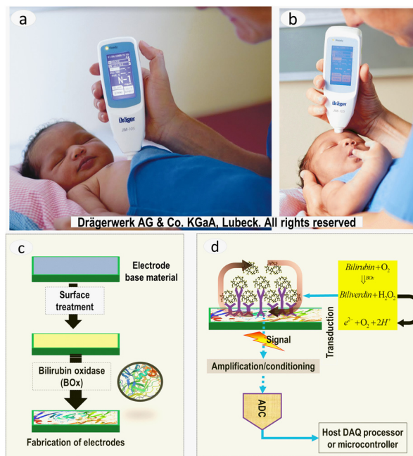
Fig. 3 (a and b) The images show newborns being measured for BR levels on the forehead (left) and sternum (right). Light is illuminated on the skin, and the reflectance is measured. The obtained information is processed and correlated with BR levels. Images were used with permission from Drägerwerk AG & Co. (c) Schematics illustrating the processes involved in fabricating and preparing bilirubin biosensors. (d) Schematic representation of chemical reactions and measurements of electrochemical response. The sensor surface with immobilized enzymes acts as an electrochemical transducer. The response measurement is achieved using an ADC for digitization and a host microcontroller/processor for data processing and acquisition.
