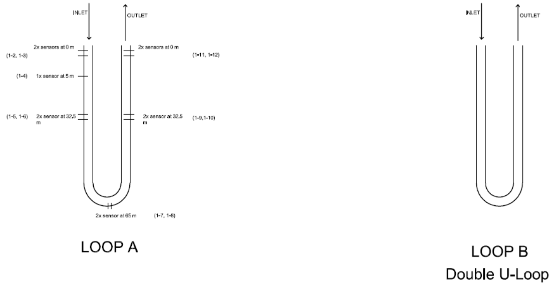
Figure B-41: Instrumentation schematic for the ground heat exchangers
