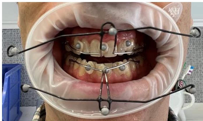
Figure A.C.1: Subject wearing motion tracking plates and 4mm hemispherical retroreflective markers attached to the mandibular and maxillary incisors and premolars.
