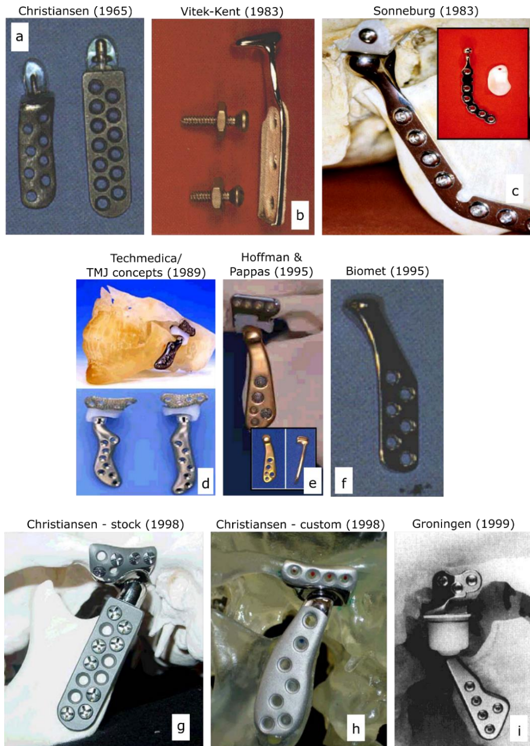
Figure 2.7: Evolution of total TMJ prosthesis designs. Shown is the Christiansen condyle prosthesis (a), the Vitek-Kent condyle prosthesis (b), the Sonneburg total TMJ prosthesis (c), the early Techmedica/TMJ concepts total TMJ prosthesis (d), the Hoffman and Pappas total TMJ prosthesis (e), the early Biomet condyle prosthesis (f), the Christiansen stock (g) and custom (h) total TMJ prosthesis and the Groningen total TMJ prosthesis (i). Further details of each system can be found in Table 2.2. Figures adapted from Driemel et al. (2009).
