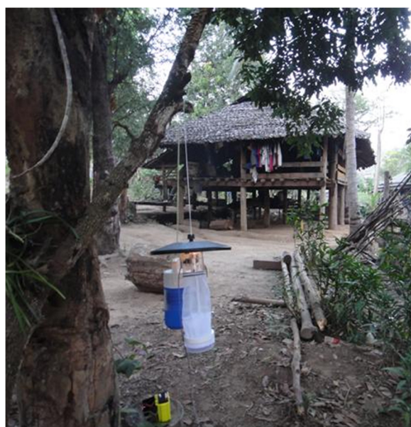
Fig. 2 CDC light trap setting. The CDC light traps with and without 1 kg of dry ice were set by hanging them in about 1.5 meter height either indoors and outdoors (10–20 meters from house), overnight (6.00 pm–6.00 am.). Mosquitoes were collected daily in the early morning
