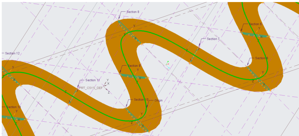
Figure 4.1 Creating river geometry with the Creo Parametric software.
