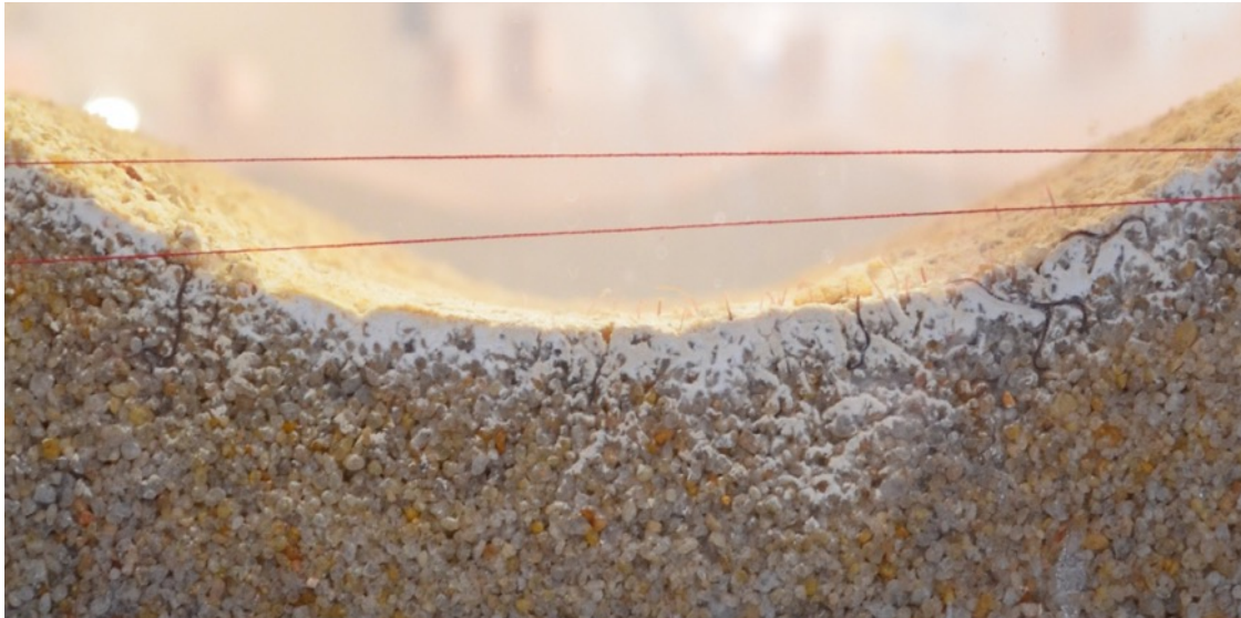
Figure 5.6: The vertical transport of clay particles in coarse sand after the seal of low permeability clay layer at the top was disintegrated by worm bioturbation
