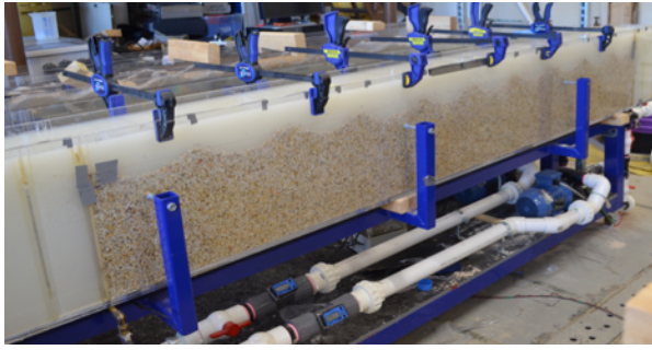
Figure 5.1: Re-circulating flume apparatus used for conducting the experiments. The inset on right shows the hydraulic conditions maintained in all the experimental flumes.
