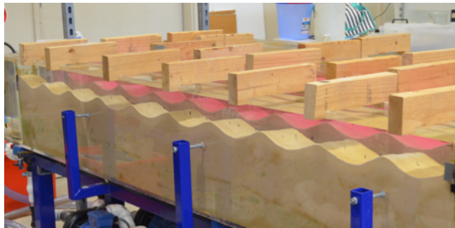
Figure 3.3: Flume set up with dune-shaped bedforms (left) and hydraulic conditions in all the experiments (right).
