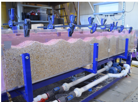
Figure 4.1: One of the experimental flumes (left) and hydraulic variables for all the experiments (right).
