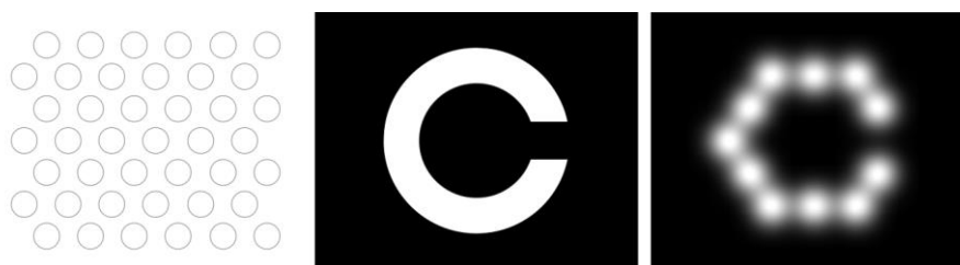
Figure 7.1: Phosphene rendering for simulated prosthetic vision using the abstract model described by McCarthy et al (2014). 137 (Left): electrode layout. (Centre): input image. (Right): phosphene rendering produced by sampling the input image at the electrode locations.
