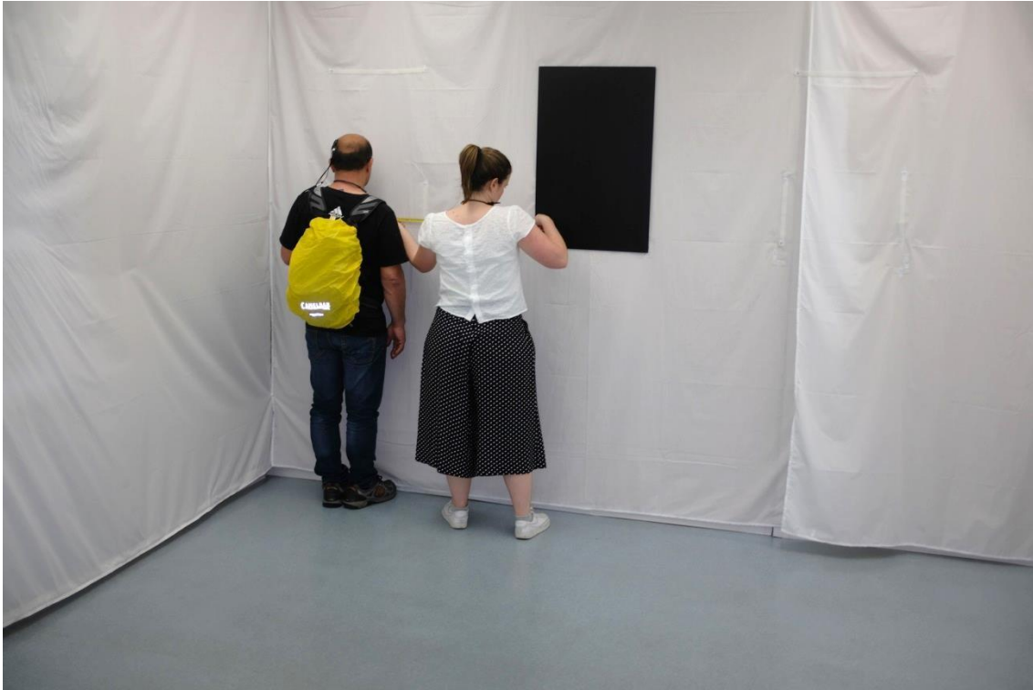
Figure 2.13: A user of the Bionic Vision Technologies 2 nd Generation Suprachoroidal Retinal Implant performs a synthetic “doorway detection” task as a measure of patient outcomes. The participant must search for a mock door (block rectangle) in a white room. A researcher (right) measures the distance from the door to the final position of the user (left).
