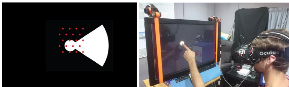
Figure 2.14: Light localisation tasks. (Left): Example of a BaLM ‘Location’ stimulus presented to a user of the Bionic Vision Australia 1 st generation suprachoroidal retinal implant in a four alternative forced-choice task. The wedge-shaped stimulus could be oriented right (shown), left, up, or down. The red dots indicate the locations in the image that were sampled to determine the electrode activity. Reused with permission from Barnes (2016). 185 (Right): Photograph of a healthy-sighted subject performing a target localisation task under stimulated prosthetic vision. The white target appeared in random locations on the screen, and the subject was required to find it and touch it with their finger. Reused with permission from Titchener (2018) [CC BY 4.0] . 17
