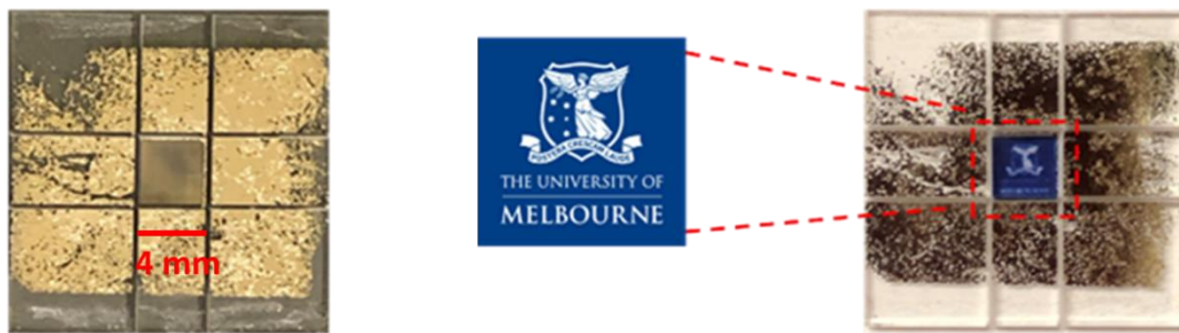
Figure 3.4 The fabricated CMY filter mosaic on the quartz substrate was cut into 4 mm x 4 mm using a dicing saw. The University of Melbourne logo on the white paper that could be seen through the filter clearly. This demonstrate the high transmission of the filter mosaic for the image sensor applications.
