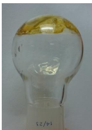
Figure S2. Physical gel obtained from the Fenton reaction conducted in the absence of the bis -functional trithiocarbonate RAFT agent.
