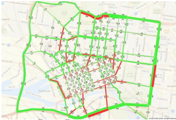
Figure 5, Melbourne's central area, user equilibrium hourly traffic flow (at-capacity roads are red colored),
