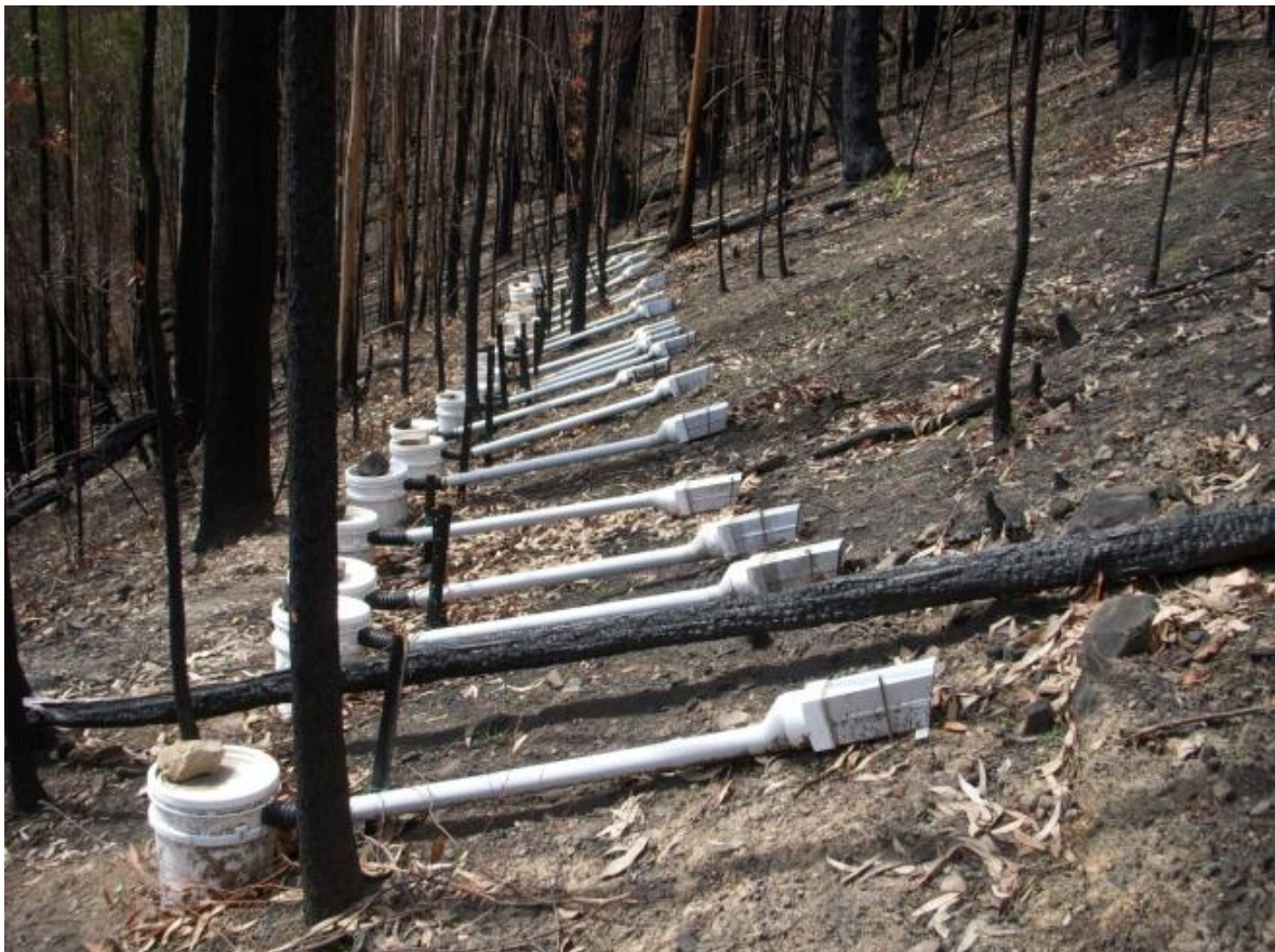
Figure 48: A transect of 20 runoff samplers on the high severity hillslope in August 2009. Samplers were located approximately 100 m from the ridge on planar hillslopes. The total hillslope length was approximately 200-300 m.
