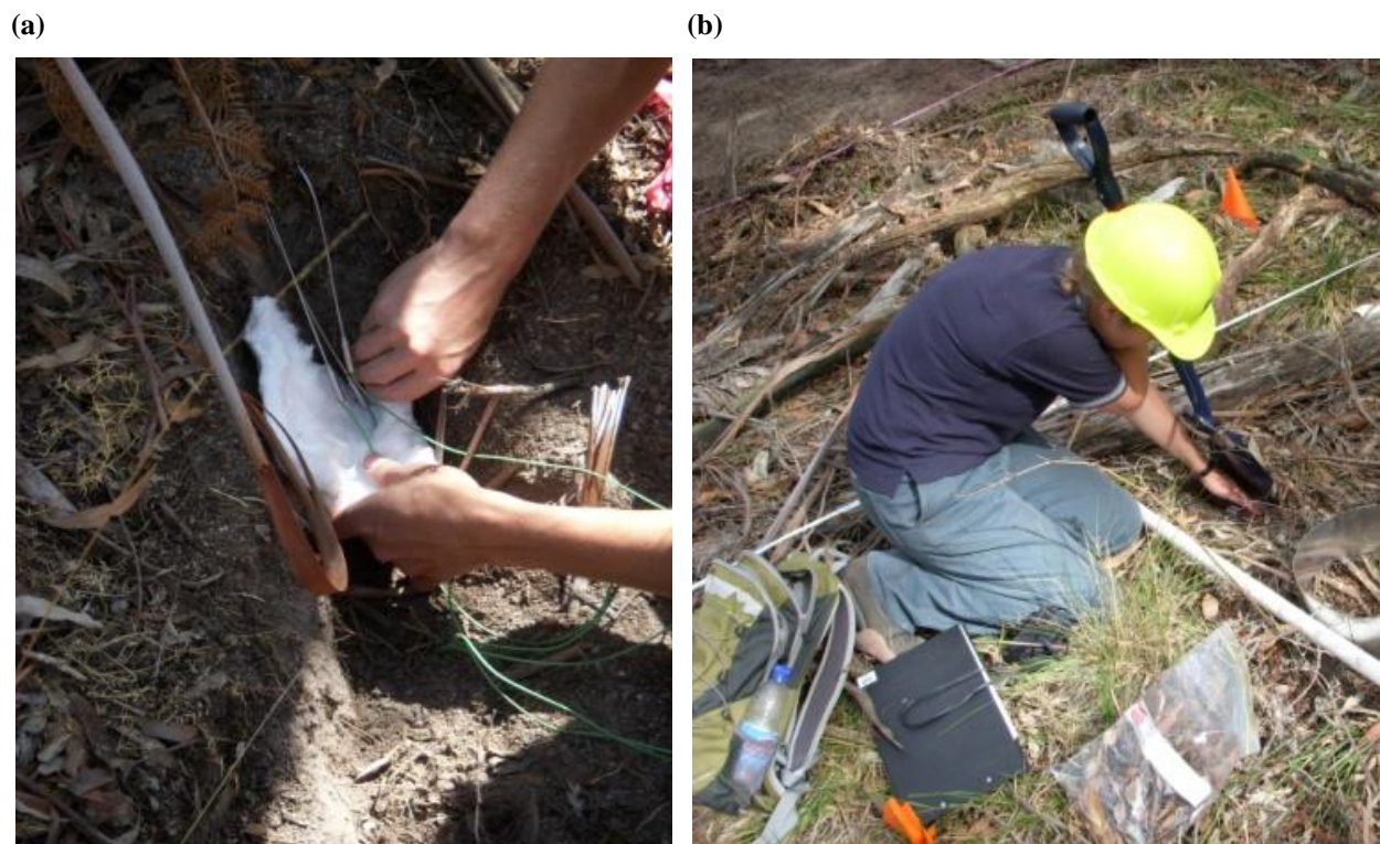
Figure 21: (a) Thermocouple installation and (b) pyrometer installation.
