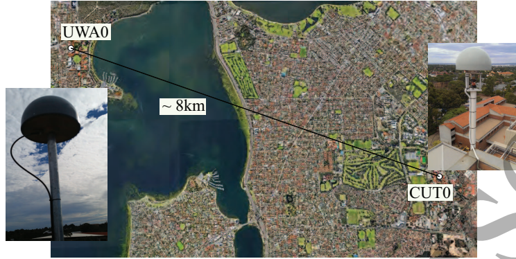
Fig. 3 Baseline CUT0–UWA0 located in Perth, Australia: [Left] UWA0 station; [Middle] baseline configuration (Map data @ 2020 Google); [Right] CUT0 station.
