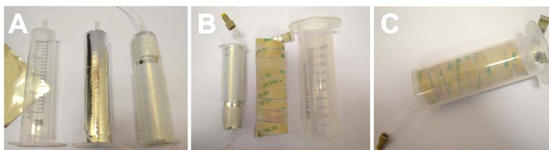
Figure 2.1.4. Simple yet highly effective flow tubular photoreactor developed by Noël and co-workers. Photoreactor is comprised of a flexible LED strip and PFA microtubing coiled around two deconstructed syringes. Cooling is provided by compressed air. Reprinted with permission from ref 156.
