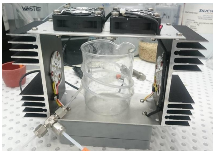
Figure 2.2.3 The tube-in-tube gas-liquid photoreactor coiled around a Pyrex® beaker and flanked by two LED (530 nm, 7 W) arrays.
