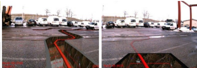
Figure 6. X-Ray view of an electricity line. Trench along the electricity line (a), Excavation Box (b) [3]
