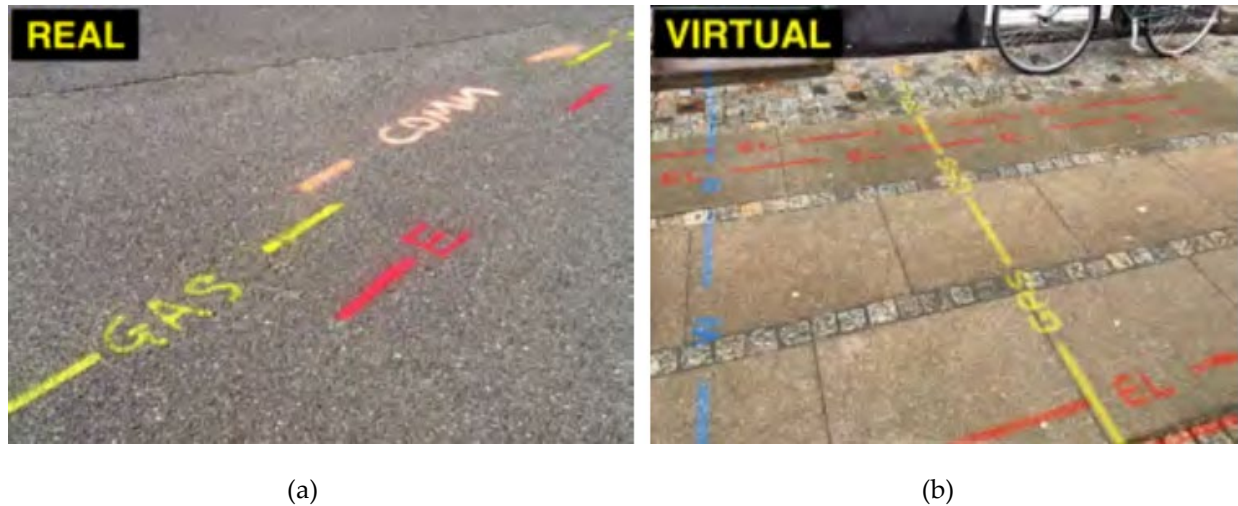
Figure 13. (a) Physical marking on street surface (b) Virtual utility marking of similar information in AR [140]
