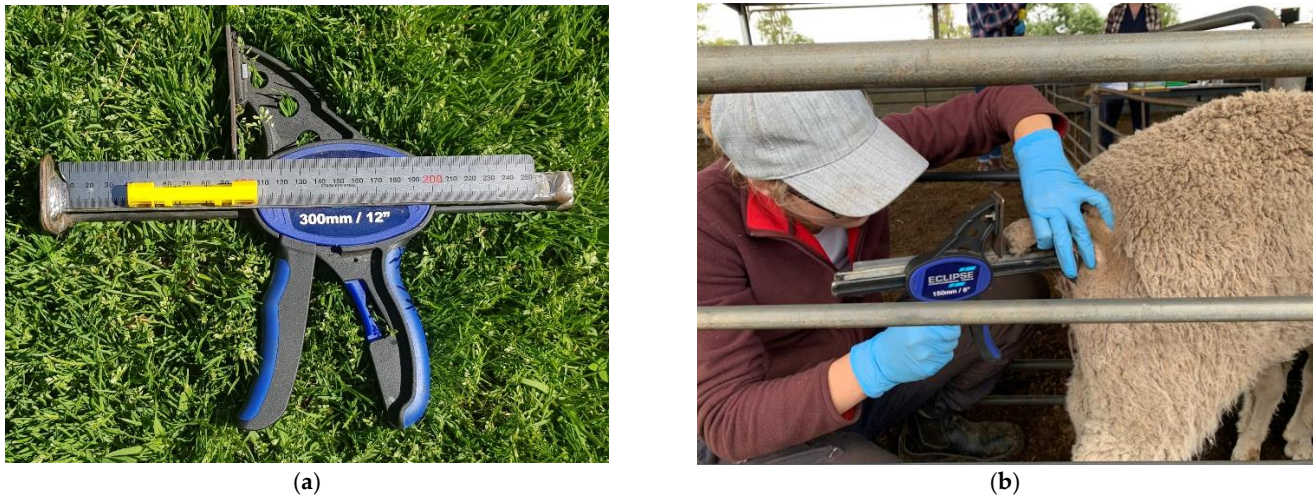
Figure 1. (a) The device created and used for the length measurement of tails. (b) The device in use on a weaner ewe.
