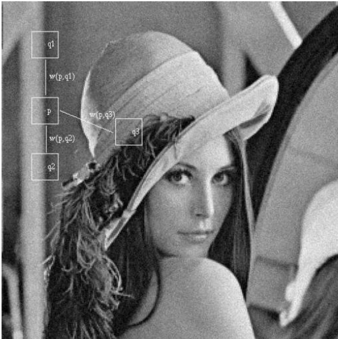
Figure 7-1 - When denoising pixel p , pixels q1 and q2 will be given greater weight than q3 because their neighbourhoods are more similar to the neighbourhood surrounding p . Adapted from Buades, et al (Buades, Morel, & Coll, 2005).
