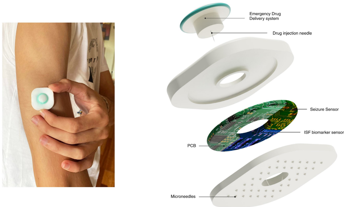
FIGURE 1 Overview of the artificial intelligence-driven closed loop device system, consisting of a continuous seizure detection sensor, a sudden unexpected death in epilepsy biomarker sensor, a processor, and an emergency drug delivery actuator. ISF, interstitial fluid; PCB, printed circuit board.
